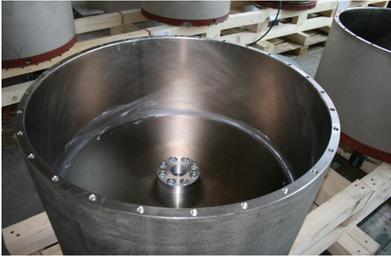
Precision honed cylinder and nickel plated cylinder and piston
